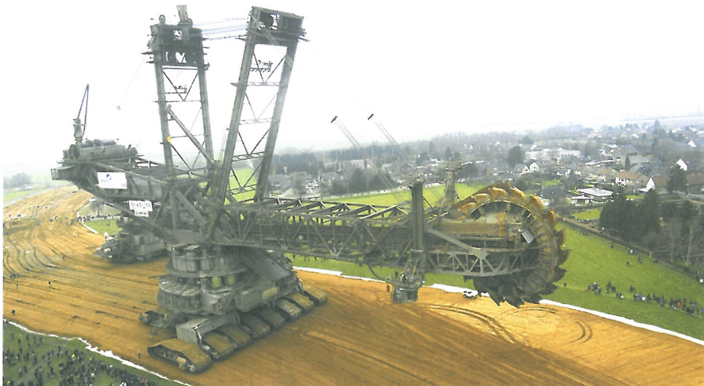
B This mining machine has large caterpillar tracks which spread its weight over a big area. The large area of the tracks spreads out the weight of the machine and makes the pressure under it smaller. This helps to stop the vehicle sinking into the soil. Look at the size of the people.
