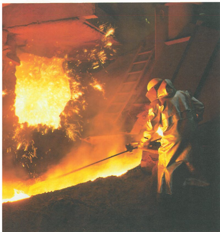
A This worker needs clothing to protect him from high temperatures and splashes of molten metal.
