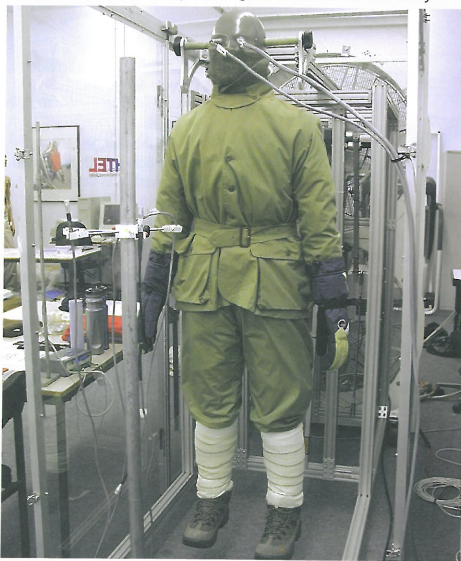
C This manikin is used to test clothing. It has heaters inside it and sensors under different parts of its 'skin'. The mechanism behind it moves it to simulate walking. In this photo the manikin is being used for historical research. It is wearing clothing similar to that worn by the 1924 expedition to climb Mount Everest.
