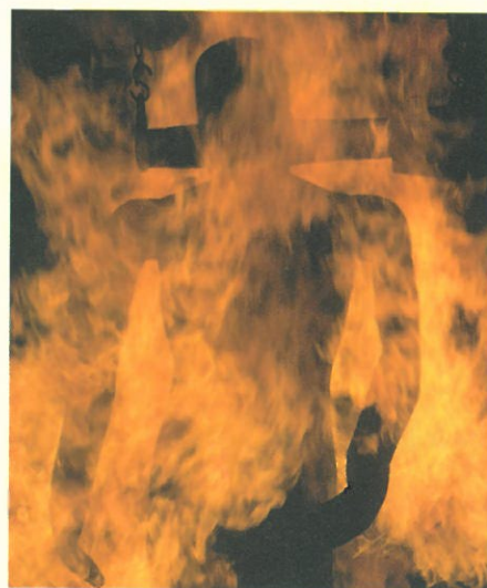
C Firefighters wear protective clothing to help them to survive in burning buildings. The manufacturers of the clothing test it using dummies like 'Pyroman'.
