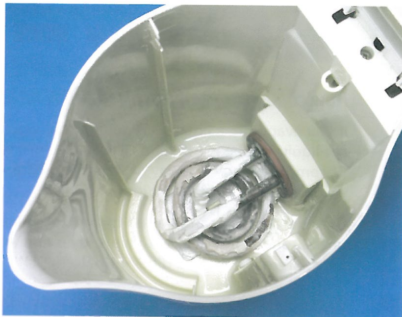
D Hard water forms scum on boiled water, and 'furs up' kettles and central heating pipes.
