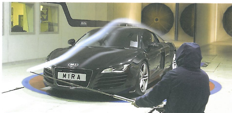
F Smoke being used in a wind tunnel to show how the air flows over a car.
