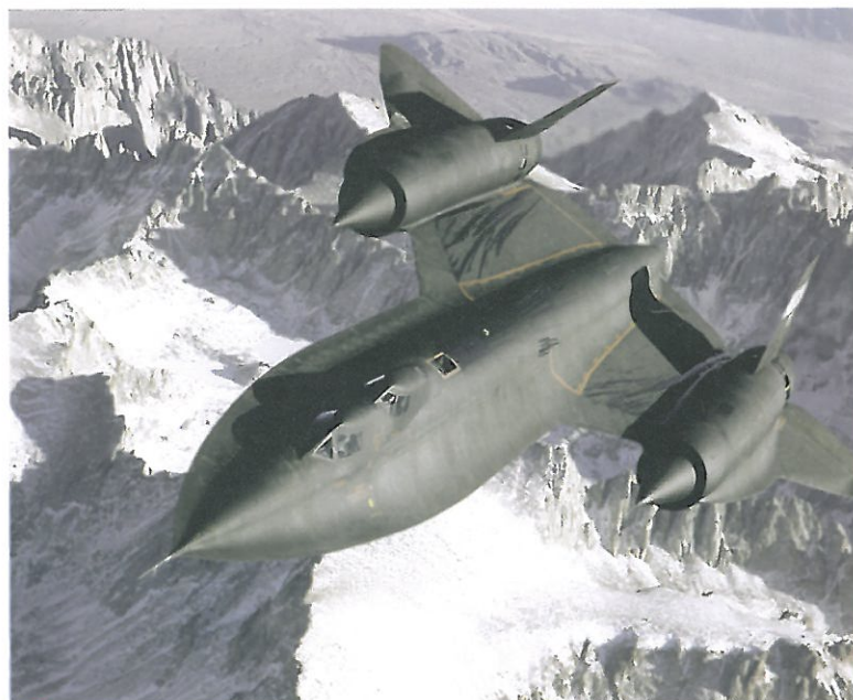
A The SR-71 Blackbird holds the record for the fastest aeroplane, with a top speed of over 2000 mph. It has a streamlined shape to make the air resistance as low as possible.
