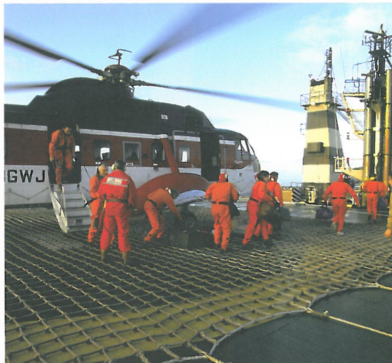
B These safety suits are designed to keep the passengers alive as long as possible if the helicopter has to ditch them in the sea. If they are worn with the correct insulating clothing underneath, a person should be able to survive for 3 hours in a cold sea.
