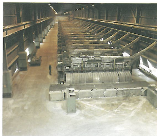
C An aluminium factory (note the size of the technician!). Enormous currents (up to 100 000 amps) are used in these factories.
