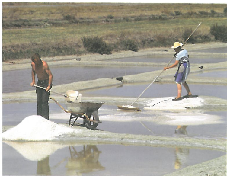
E Collecting salt made from the evaporation of sea water in France. This is called the salt-bed method.
