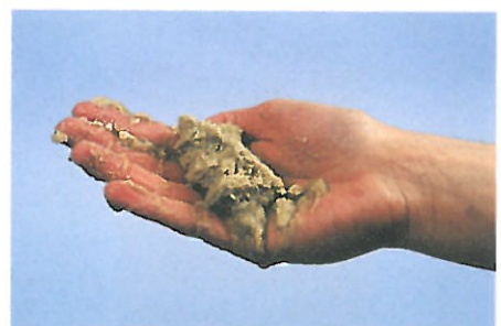
B When wet grains of sand are squashed together, water runs out and the grains of sand stick together.
