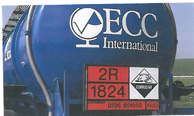
E A Hazchem warning symbol is always displayed on tankers carrying acids.
