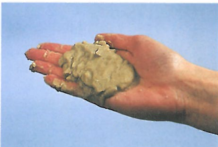
B When wet grains of sand are squashed together, water runs out and the grains of sand stick together.
