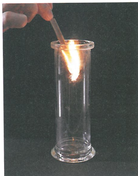
D A glowing splint put into a jar of oxygen.
