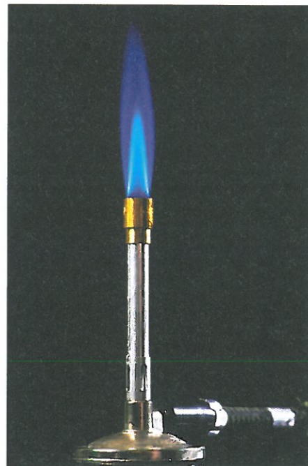
A This Bunsen burner uses natural gas. When the gas burns the energy stored in the gas heats up the surroundings.
