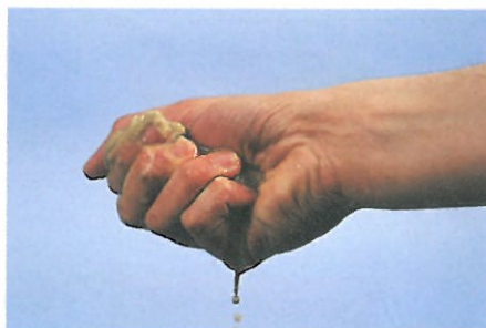
B When wet grains of sand are squashed together, water runs out and the grains of sand stick together.
