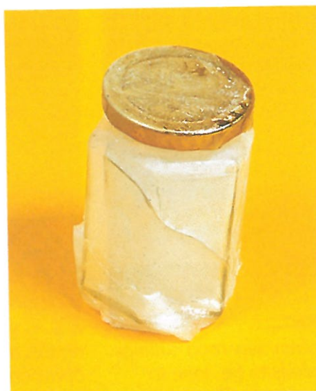
E Water freezing inside this jar has expanded and split it apart.
