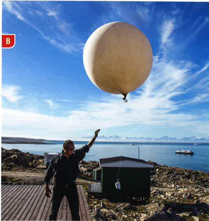
▲ Four times a day, weather balloons are launched from six sites in the UK. The little package collects and transmits data.
