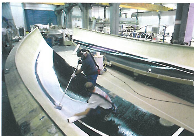
E Making a composite yacht. Mats made from woven fibres are put onto a mould, and liquid resin is applied. This will set to form a rigid shape when it is heated.
