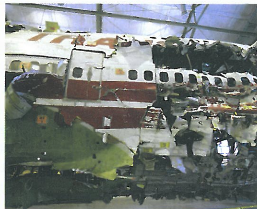
A Air accident investigators piece together bits of crashed aeroplanes to help them to work out why the crash happened.
