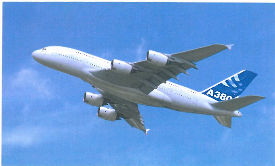
C An Airbus A380 can carry over 850 passengers. It is made of aluminium alloys and composite materials such as carbon-fibre reinforced plastic and glass-fibre reinforced plastic.
