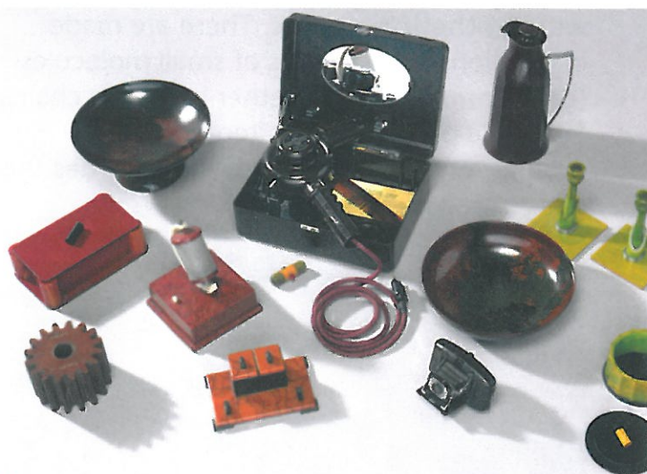
A Bakelite was the first widely used synthetic polymer. It was invented by Leo Baekeland (1863–1944), and started selling in 1909. It was used to make many different things, including electrical switches, cups and even propellers!
