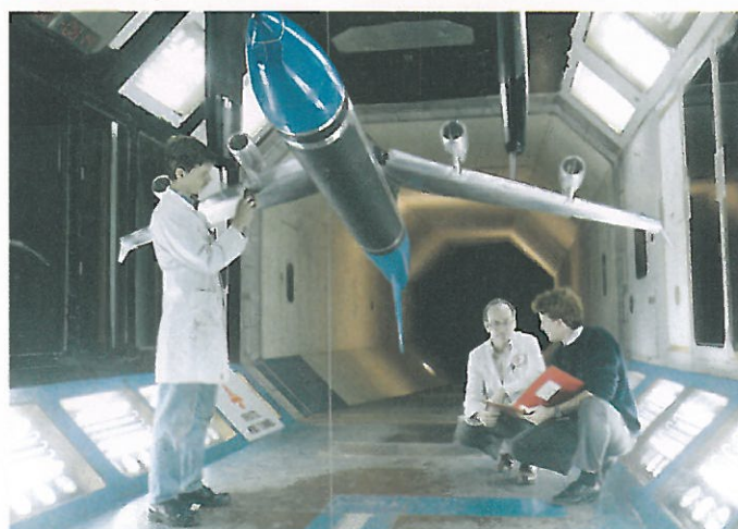
C Scale models of aeroplanes are tested in wind tunnels to check how accurate computer models are. The wind tunnel blows air past the model, which is fitted with sensors to measure the forces on it and the air pressure around it.
