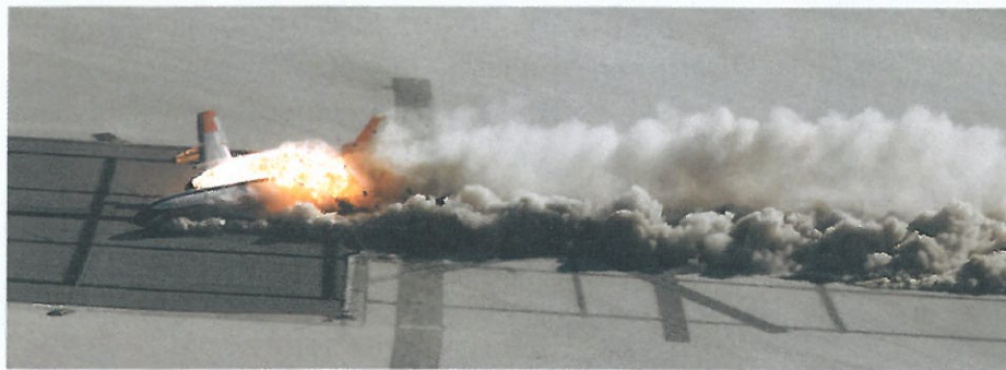
E This aeroplane was landed by remote control. Stakes were put in the ground to deliberately damage the wings and fuel tanks.
