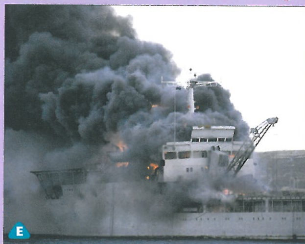
The Sir Galahad burned fiercely when the ship was attacked in the Falklands War in the 1980s. The explosive impact broke the aluminium into small pieces, which then reacted violently with oxygen in the air.
