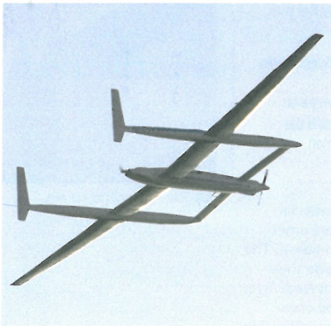
F Voyager made the first non-stop round the world flight in December 1986. Its flight lasted just over nine days. Most of Voyager was made from composite materials.
