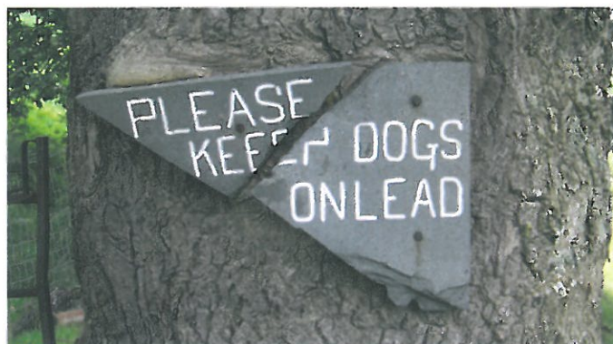
A This slate sign is fixed to the tree by nails. As the tree grew wider, the slate broke.
