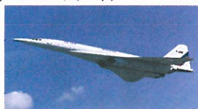
▲ The Tu-144 holds the record for the fastest passenger aircraft. It could travel at around 2500 km/h. Like most aeroplanes, it has a streamlined shape to reduce its air resistance .
