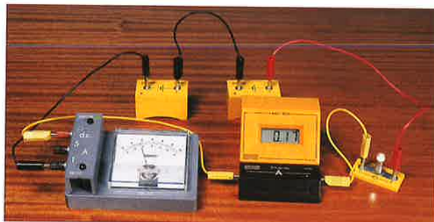
Figure 18.4 Ammeters measure electric current, in amps (A). There are two types: analogue (on the left) and digital (on the right).
