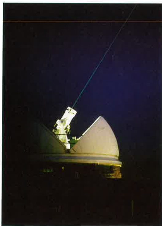
Figure 13.1 A laser beam is directed into space from the Royal Greenwich Observatory (Sussex, UK). The beam reflects off the Moon or a satellite in space. The reflected beam is detected, and the exact distance to the Moon or the satellite can be calculated.
