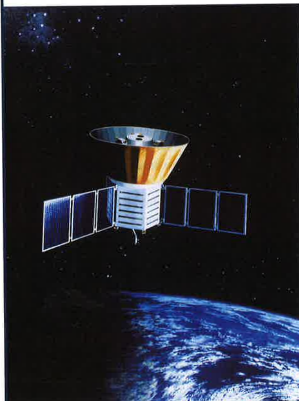
An artist's impression of the Cosmic Background Explorer in space. This spacecraft measured the temperature of space by detecting the radiation left over from the Big Bang. The gold-coloured 'skirt' shields the temperature sensors from heat from the Sun and Earth.
