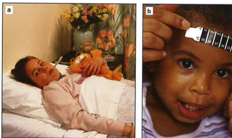
Figure 10.1 Measuring human body temperature using a a liquid-in-glass thermometer and b a liquid-crystal thermometer.
