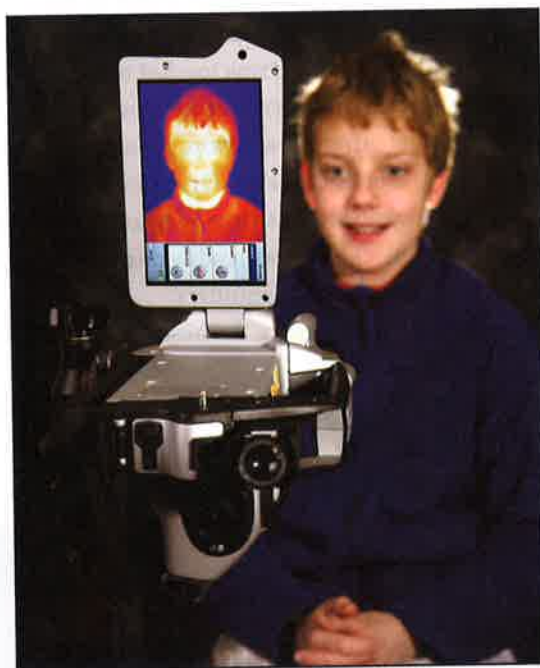
Figure 11.11 Using an infrared-sensitive camera. Slight variations in body temperature show up as different colours. Cameras like this are used in medicine to detect skin disorders and infections.
