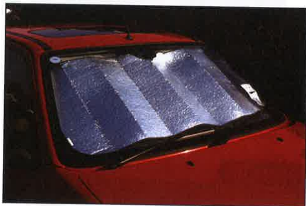
Figure 11.12 A sunshield reflects away unwanted radiation, which would otherwise make the car unbearably hot.
