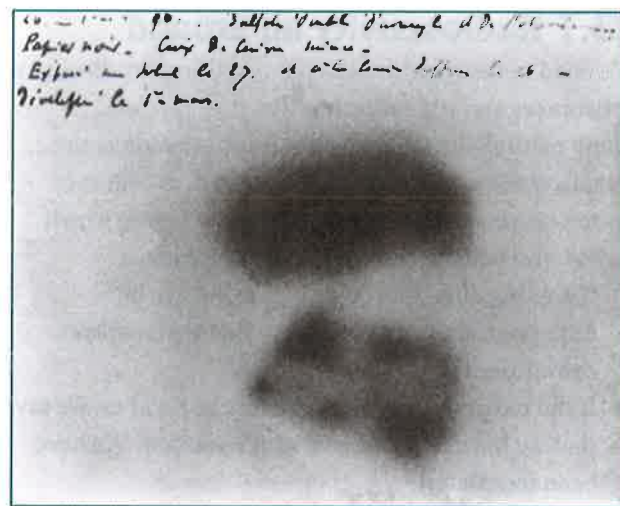
Figure 23.4 One of Henri Becquerel's first photographic records of the radiation produced by uranium. The two black blobs are the outlines of two crystals containing uranium. To show that the radiation would pass through metal, he placed a copper cross between one of the crystals and the photographic film. You can see the 'shadow' of the cross on the photograph. The writing is Becquerel's; the last line says 'développé le 1er mars' – developed on 1st March (1896).
