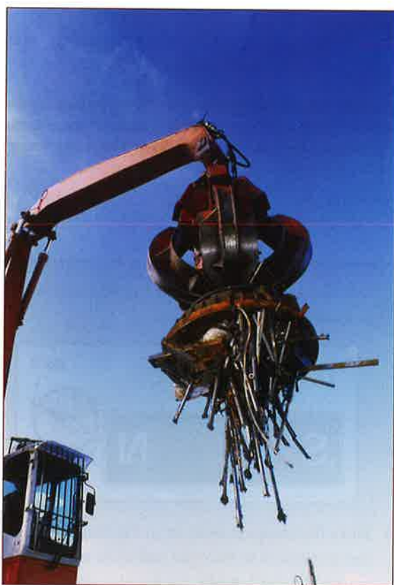
Figure 16.9 Using an electromagnet in a scrapyard. With the current switched on, a steel object or pile of scrap can be lifted and moved. Then the current is switched off to release it.
