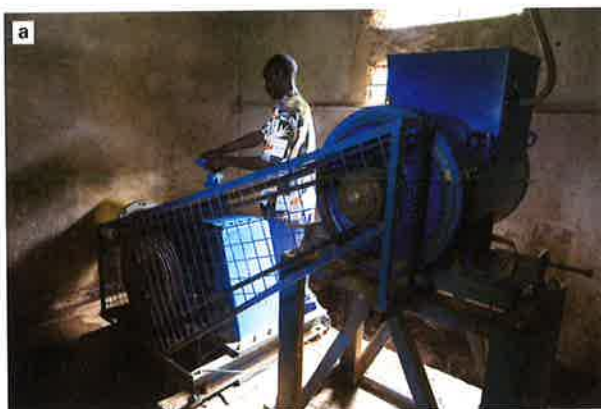
Figure 21.1 The production and use of electricity in Tungu-Kabiri, Kenya. a Water from a dam is fed through the wall in the yellow pipe to the turbine on the left. A rubber belt transfers the rotation to the generator at the top. The operator is opening the valve to control the flow of water. b Welding equipment in use in the workshop in Tungu-Kabiri.
