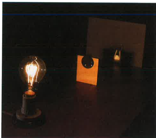
Figure 13.17 Forming a real image of a light bulb using a converging lens. The image is upside down on the screen at the back right.
