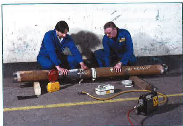
Figure 23.15 Checking for faults in a metal pipe. The engineers are checking that no radiation is escaping from the pipe. The gamma source is stored in the black box in the foreground, but can be pushed through the long tube along the pipe to reach the part to be checked.
