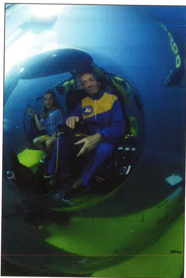
Figure 5.9 This underwater exploring vehicle is used to carry tourists to depths of 600 m, where the pressure is 60 times that at the surface. The design makes use of the fact that spherical and cylindrical surfaces stand up well to pressure. The viewing window is made of acrylic plastic and is 9.5 cm thick.
