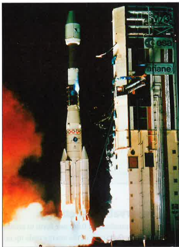
Figure 6.6 This giant rocket uses rocket motors to lift it up into space. Each rocket motor burns about one tonne of fuel and oxygen every minute to provide the energy needed to move the rocket upwards.
