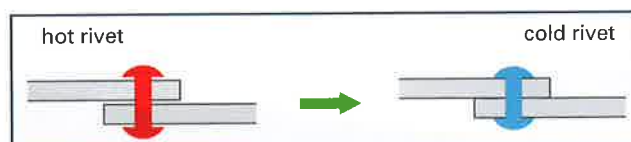
Figure 10.9 Joining two metal plates using a rivet.
