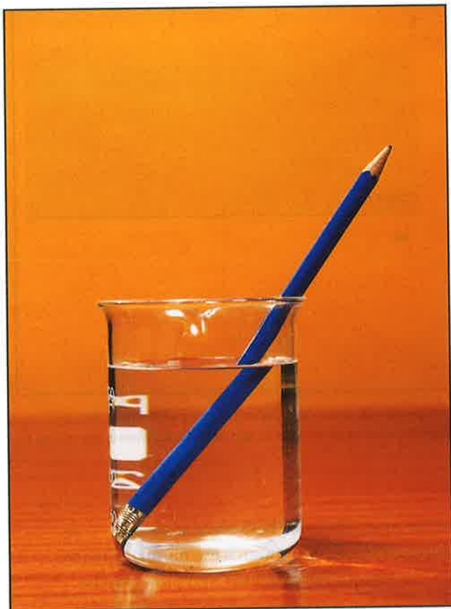
Figure 13.7 The pencil is partly immersed in water. Because of refraction of the light coming from the part of the pencil that is underwater, the pencil appears broken.
