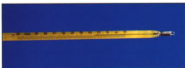
Figure 10.4 A modern Celsius-scale liquid-in-glass thermometer, with a fixed quantity of mercury sealed in a glass tube.
